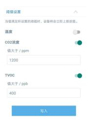
Method 2: Open the Toolbox software on the computer and enter the configuration interface, and configure the threshold value of the corresponding sensor on the page of "Device Settings" Basic Information Threshold Settings".
