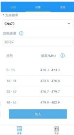
Method 2: Open the Toolbox software on the computer and enter the configuration interface, select the support frequency and enable the corresponding channel on the "Set up> Channel" page.
