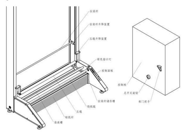
1. Turn the control cabinet knob fixed to the wall clockwise, and the green indicator light on the equipment turns on;
